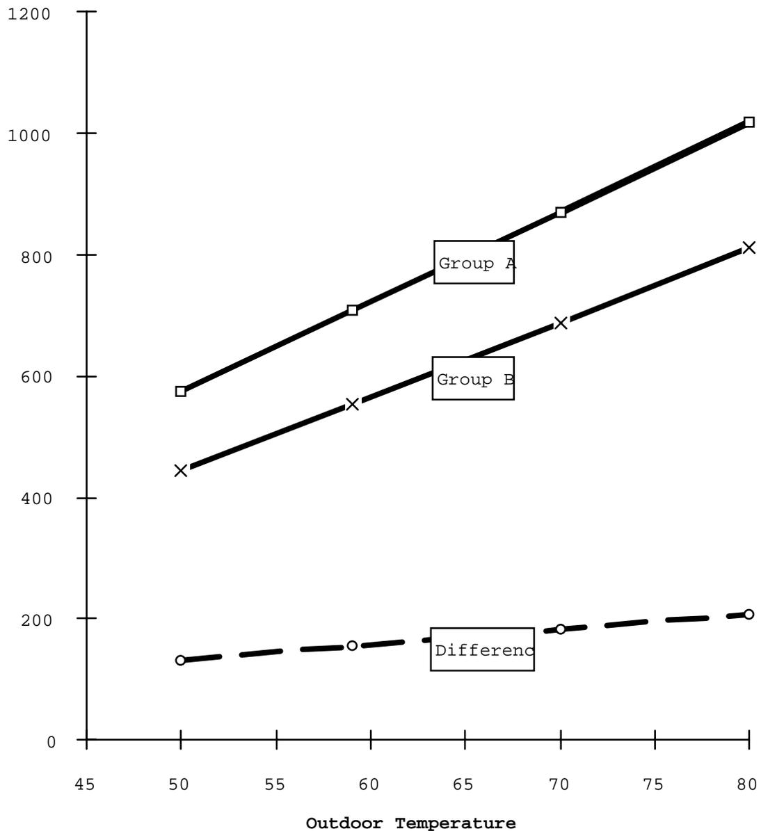
Clearly the energy consumption of these refrigerators is dependent on outdoor temperature. In addition, the difference in consumption (savings) decreases as the outside temperature drops. Figure 2 shows the projected annual savings at an average outdoor temperature of 59°F (the weighted average temperature for PG&E's residential customers). Also shown is the 95% confidence interval for the metered difference.
